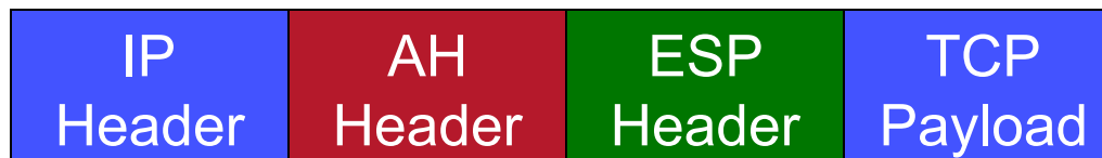
Packet format with AH and ESP
