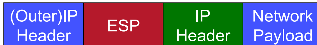
IPsec tunneled mode packet format
