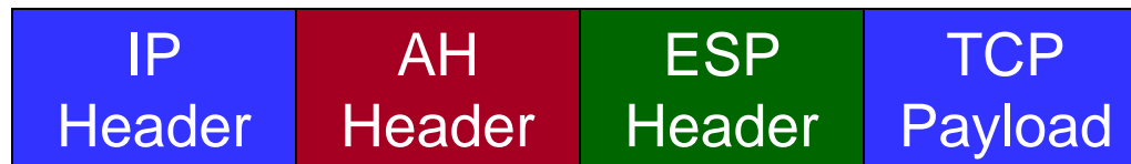
Packet format with AH and ESP
