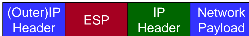
IPsec tunneled mode packet format
